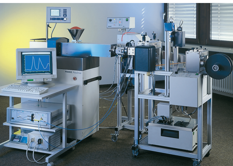
Twin-screw extruder with near-infrared spectrometer.
